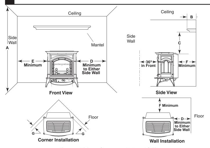
Figure 5 - Minimum Clearance to Walls and Ceiling
